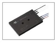
**ACP's** 100 GHz 2 Channel OADM utilizes thin film coating technology and proprietary design of non-flux metal bonding micro optics packaging to achieve optical add and drop at the ITU wavelength. It provides ITU channel center wavelength, low insertion loss, high channel isolation, wide pass band, low temperature sensitivity and epoxy free optical path. It can be used for wavelength add/drop in telecommunication network system. All AC Photonics' products are Telcordia qualification tested.
